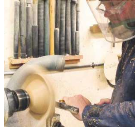
▲ Pic.21 It's absolutely imperative that you wear personal protection equipment when turning, especially on pieces such as this. Place a firm grip on the tool and make sure your hand is always behind the toolrest
